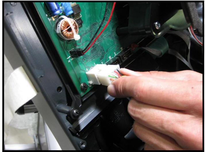
Step 6. Disconnect the 12-pin serial connector from the display.
